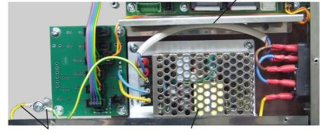
connect the earthing wires
