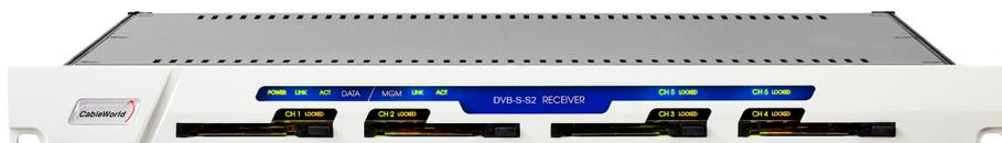
CableWorld’s latest receivers are available in several versions to satisfy user demand. The fully equipped 19–inch rack contains six tuners which are for demodulating DVB-S/S2 and DVB-S2X signals, and four CI slots (Conditional Access Module sockets). The CI slots are assigned to the first four tuners, the fifth and the sixth tuners can be used for reception of free-to-air services. The device provides both ASI and IP (UDP/IP or RTP/IP, MPTS or SPTS) outputs.
