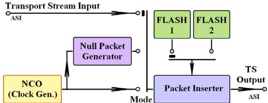
Block diagram of the CW-4881 TS Generator & Inserter
