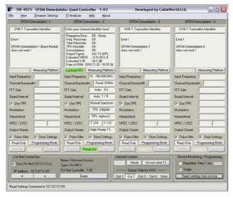
Now as the demodulator is tuned you can inspect the parameters of the modulation and reception:
