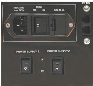
The ACTIVE COMBINER is built with the most advanced GaAs hybrids which are cooled with an internal high lifetime blower. The values of the internal supply voltages (+24V, +5V) and the temperatures of the 6 hybrids are measured by microcontroller, which can be contacted via the CW-Bus of the CW-4000 system. In headends not equipped with this bus, the same function is available from the serial port of the PC, by using a CW-4059 DEMO CABLE and the SW-4076 software.
